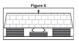
After each time the load is lifted, slowly empty the Lift Bag lowering the load onto the safety supports.
