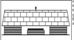
mm (2.76") space between the ground and the object to be lifted, build a firm foundation leaving just enough space to insert a non inflated bag onto the foundation and under the load. The foundation must be undivided without any gap under the Lift Bag (**Figure 5**). Add safety supports to each side of the Lift Bag/s as the load is lifted (**Figure 5**) to support it in the event the Lift Bag or inflation system fails.
