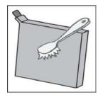
Clean the Lift Bag surface with a brush with hard bristles moving the brush in all directions. Never use a sharp brush that might damage the Lift Bag. After brushing off the dirt, use a brush to wash off any remaining oil or dirt with a light solution of warm water and a dish washing detergent using the brush (**Figure 13**).
