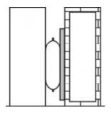
Lift Bags also be used to separate or move objects. To prevent damage care must be taken if an object has thin walls which could be bent or broken by the pressure. The Lift Bag should be positioned against a rib, a pillar, or another strong and rigid section. Otherwise insert a fiberboard between the Lift Bag and the object to increase the surface area (**Figure 12**).
