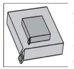
In order to increase lifting height it is also possible to use two air bags. Place the smaller one in the middle and on top of the larger one, with the inflation nozzles pointed away from the load (**Figure 7**). Never stack more than two air bags under a load.
