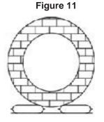
Cylindrical objects of great size such as tanks don't admit lifting by a single Lift Bag. If the object is not firmly fastened it will roll away when the Lift Bag begins inflating to its typical spherical form. Cylindrical objects must be lifted using two Lift Bags, one at each side of the object. The inflation must be controlled to permit equal coordinated lifting (**Figure 11**).
