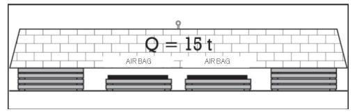
**Figure 8** shows two Lift Bags, placed next each other under a 15 ton foundations. The first Lift Bag can lift 8 tons, the second 12 tons. Neither of the bags can lift the load of 15 tons alone, however, together they are able to lift up to 20 tons.
