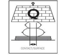
The lifting height can be increased by stacking Lift Bags (**Figure 9**). If the lifting height of one Lift Bag is 18 cm max and of the other 22 cm, both together and fully inflated can achieve the lifting height of 40 cm.
