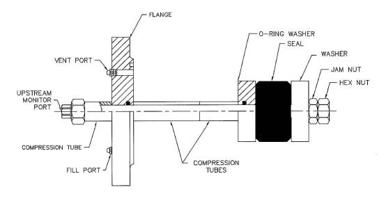
Figure 3. High Lift Flange Weld Test Plug. 4" through 8" Plug Sizes. Shown in WP Configuration
