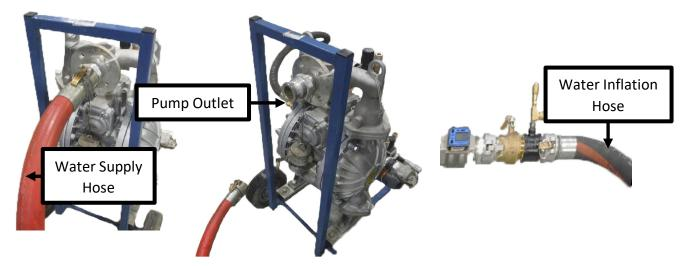
**3.** Verify that the Water Pump Outlet Hose drains into a tank or area that can collect the water pumped out of the plug. Zero the batch counter to track the output.
